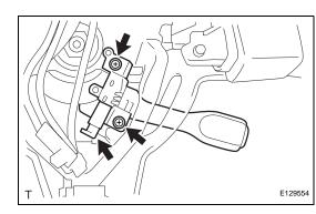
If the result is not as specified, replace the cruise control main switch.
